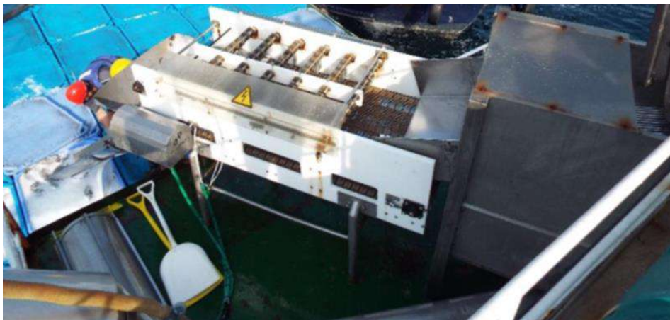
Figure 9. Optimar stunner with a dewatering unit (right) used on the Turkish coast to stun seabream and seabass (Optimar, 2024).
