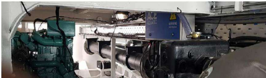
Figure 8. Example of an electric tube stunner on deck ( Ace Aquatec, 2024 ).
